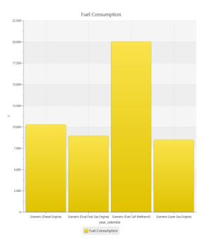
Figure 6: Fuel Consumption of different primary energy converter
